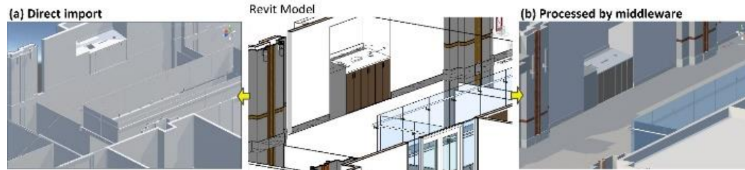
215 Figure 3. Results comparison between different model preparation approaches: (a) direct import 216 of FBX file exported from Revit; (b) processed by third-party middleware before importing
