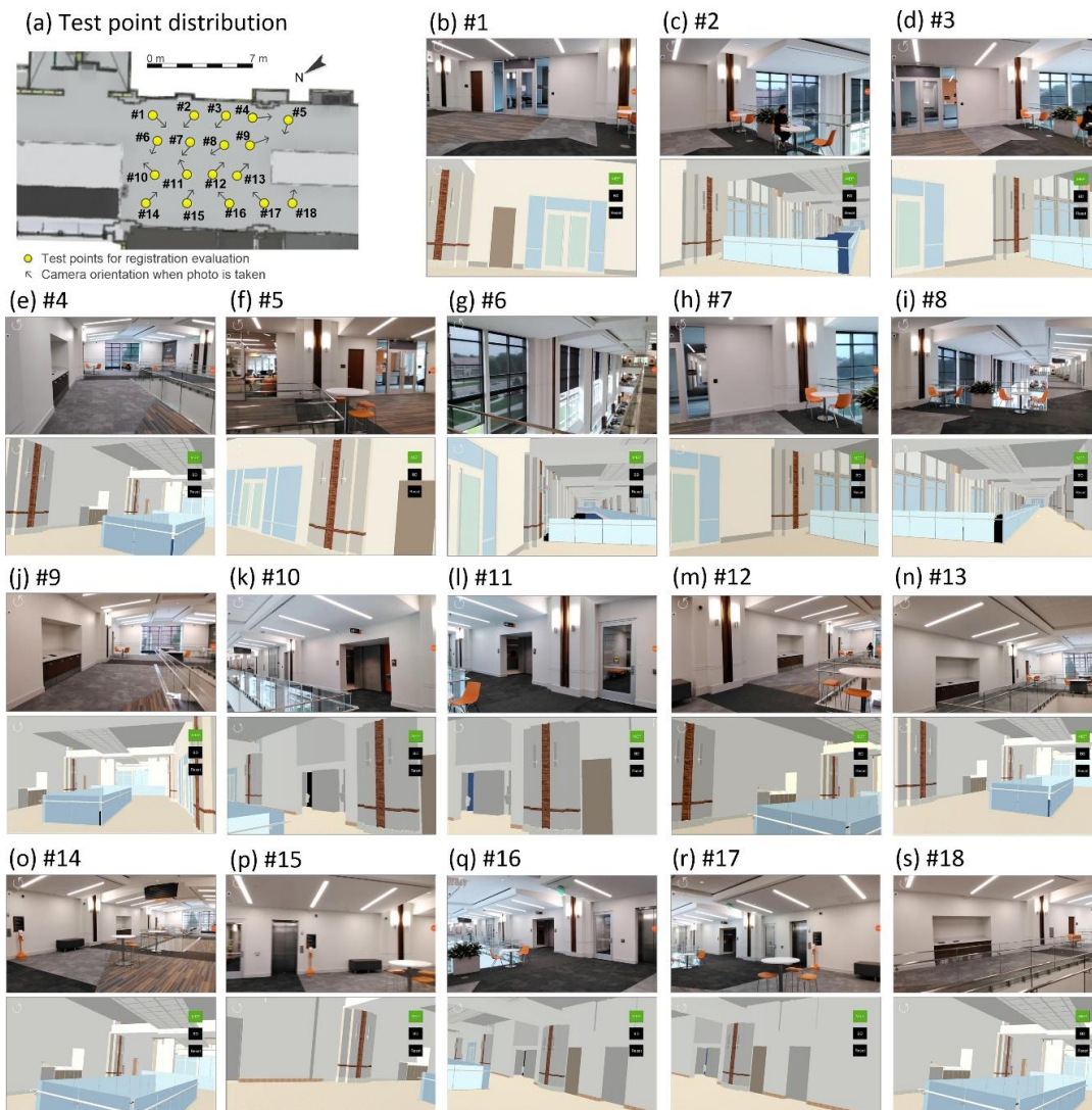
282 283 Figure 4. Setup and results of registration evaluation experiments: (a) distribution of test points in 284 the experiment site; (b)~(s) image pairs showing level of alignment between virtual and real 285 content after registration at each test point
